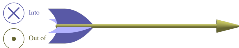
Figure: The convention we use to represent the third dimension relative to some two-dimensional figure is to use a dot to represent "out of" and an \times to represent "into". A useful way to remember this is with an arrow; if it points at you it is a dot and away an \times .
